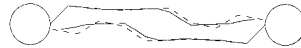
Figure 23. Crack paths for the coarse (dashed line) and fine (solid line) meshes
